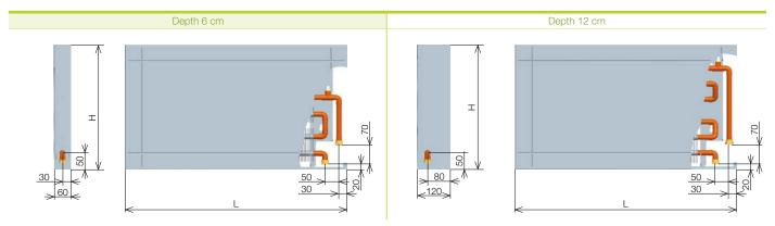
OKN is available in right or left version. The connecting side must be indicated in the order. In the schematic representations the dimensions are expressed in mm.
